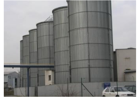
Fig. 6 - Aging of beads
