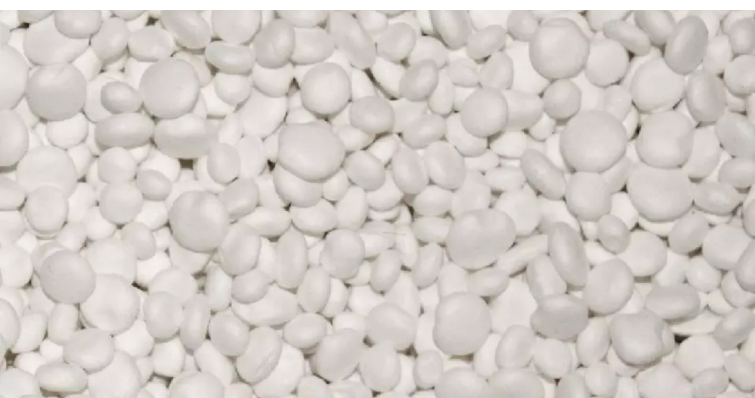
Fig. 13 - Raw material for the production of EPS
