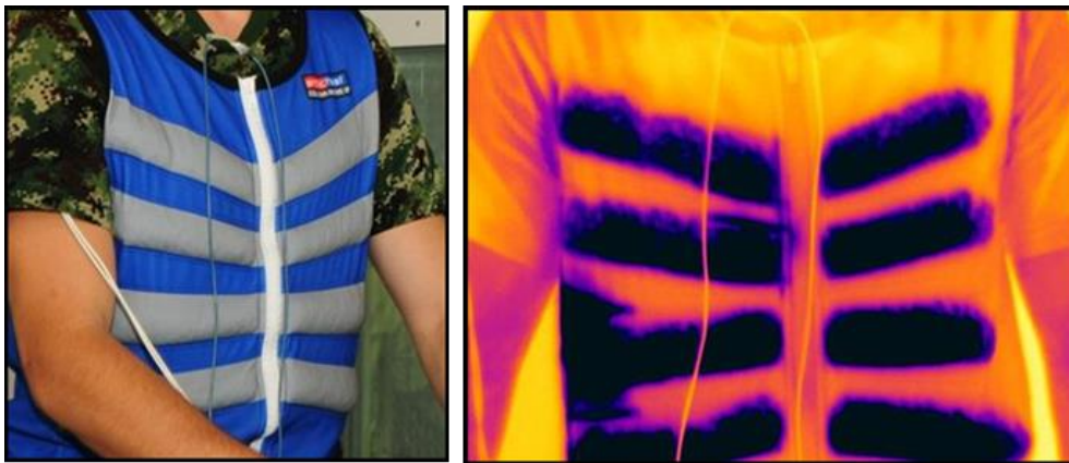
Figure 1. Snapshot vest recorded with standard and thermal imaging camera, after 30 minute of exercise
