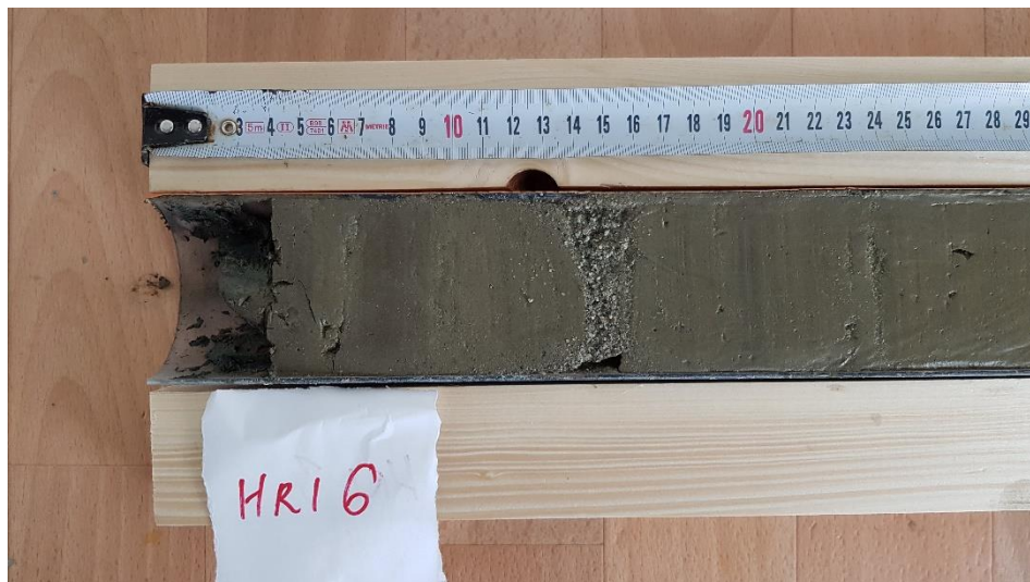
Fig. 2 Photo documentation of the drill core from the Hričov dam with a visible change in the granular fraction of sedimentation
