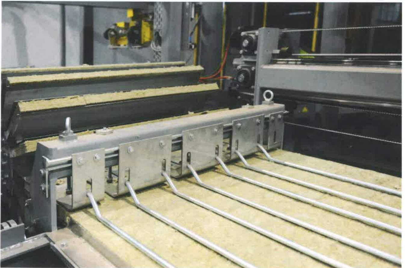
Photo 2 - Thermal insulating pads prepared at carousel
