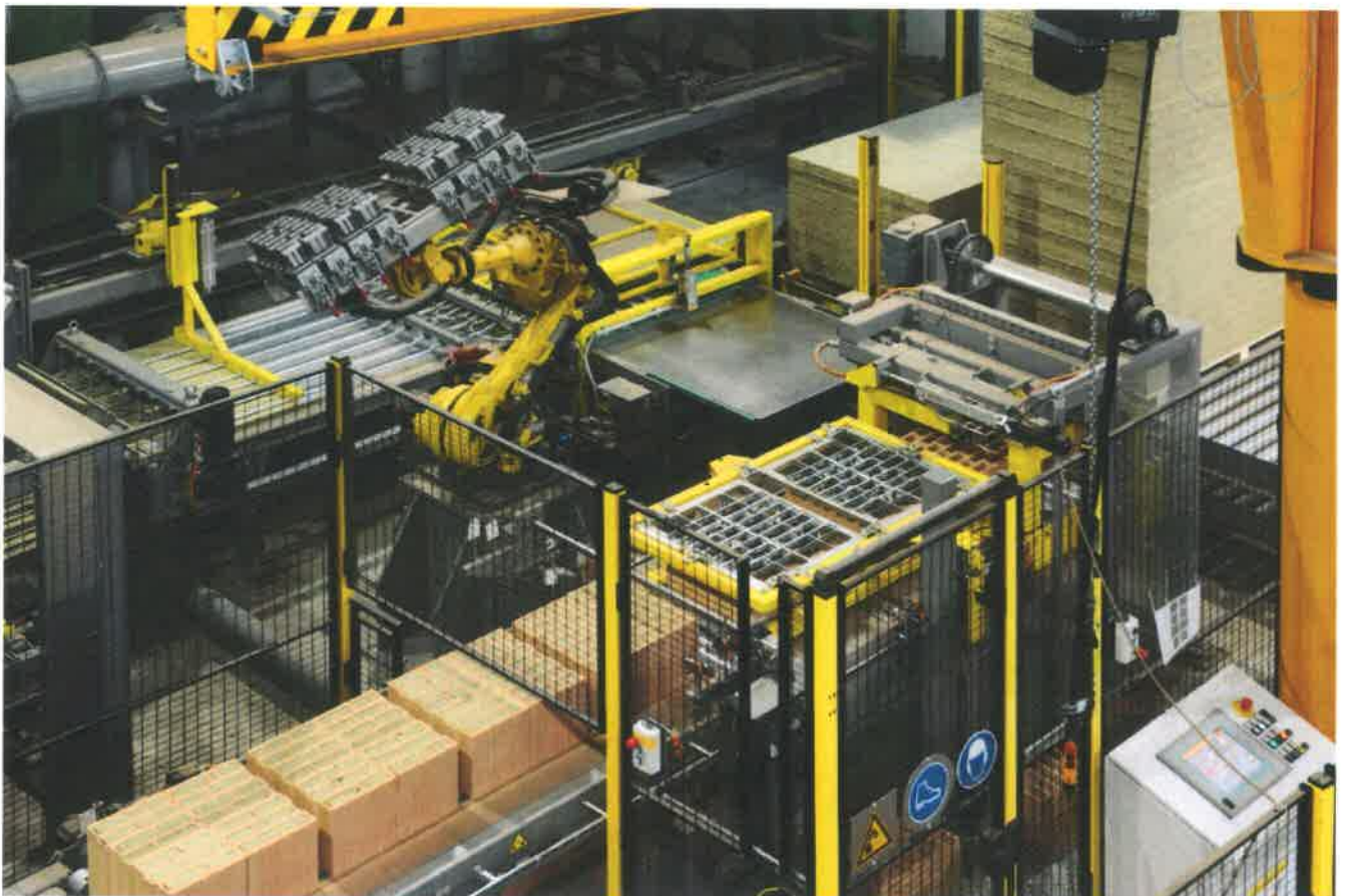
Photo 4 - Inserting thermal insulation into brick blocks
