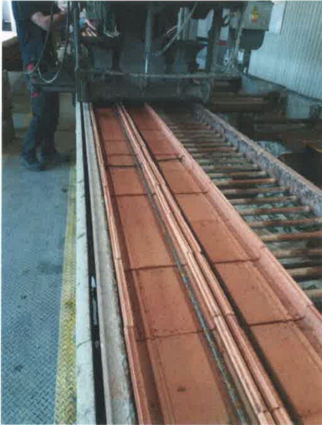
Photo 2 – Moistured U-shaped masonry units before concrete placement
